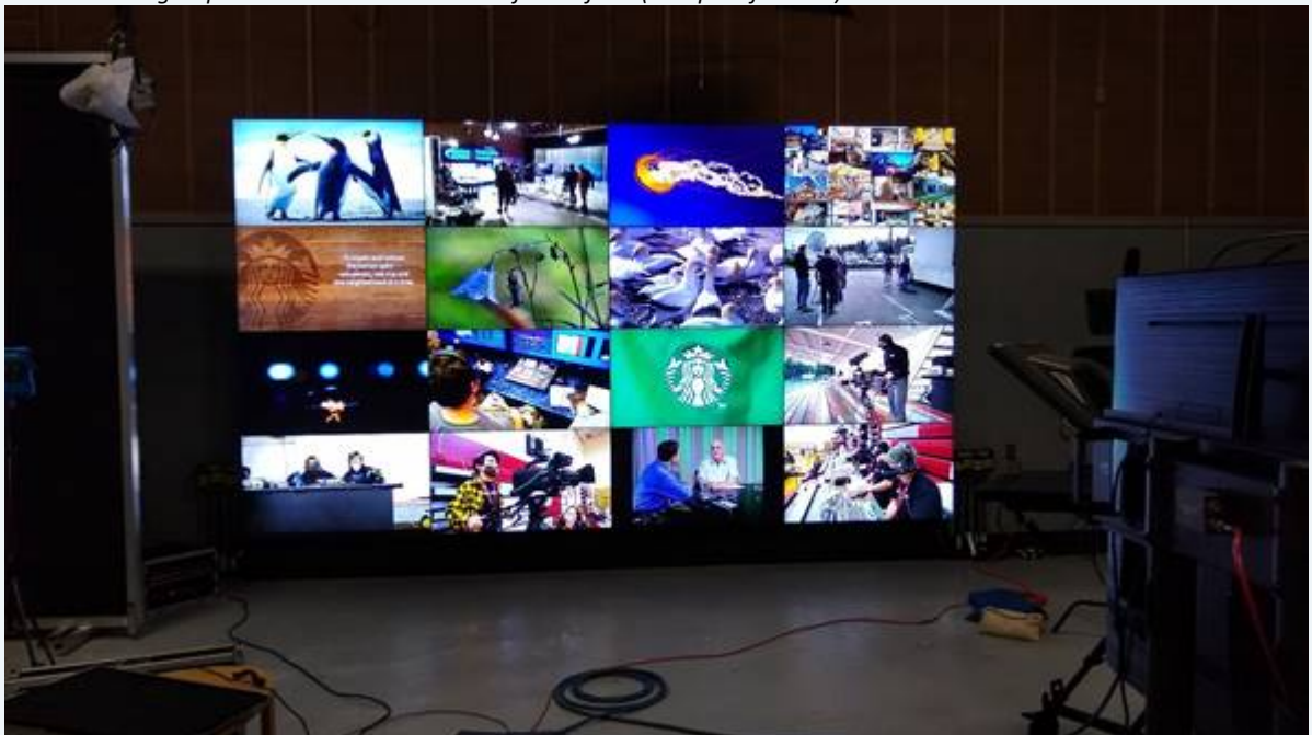
Installed 16' x 9' video wall, donated by Starbucks through Utter & Associates, displaying 16 different pictures, video clips, and live video feeds.
